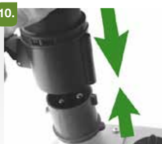
7. Insert the suction pipe (B) into its housing and tighten the handle (A).
